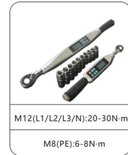
**NOTE:** Use a torque wrench to tighten the screws/nuts with reference to the torque ranges provided above.
