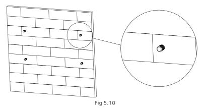
$\textbf{Notice:} \ \ \textbf{Expansion bolt should be installed on solid walls with at least 100mm thickness.}$
